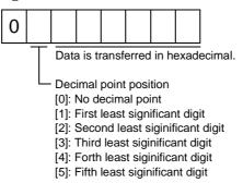
By way of example, here is described how to process the set data when a value of "15.5" is sent. Since the decimal point position is the second digit, the decimal point position data is "2". As the data to be sent is hexadecimal, the decimal data is converted into hexadecimal. 155 9B
